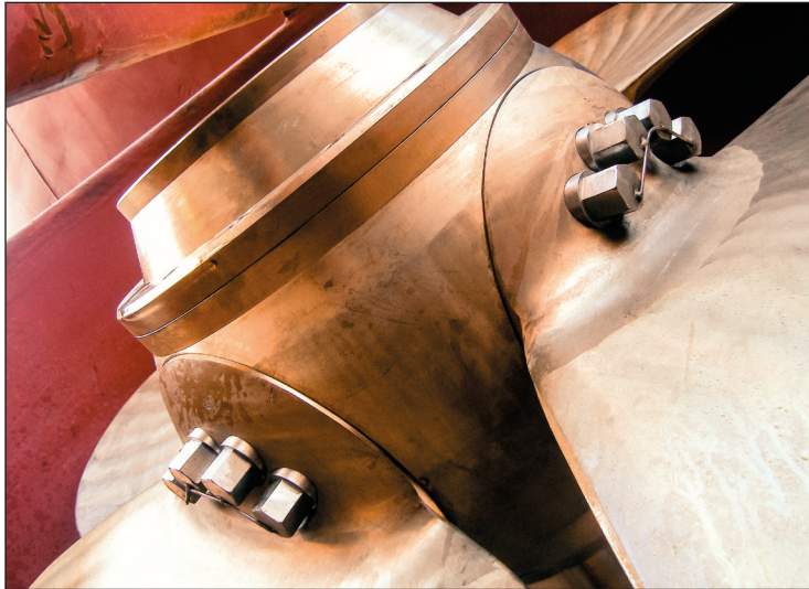
Figure 1.10 Close-up of a variable pitch propeller showing how each blade can change its pitch
