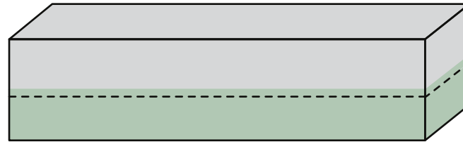
Figure 1.12 - Draught increases as water density reduces.
