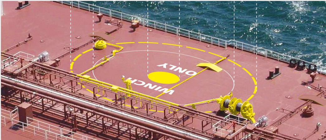
Obstructions in this area should be highlighted
