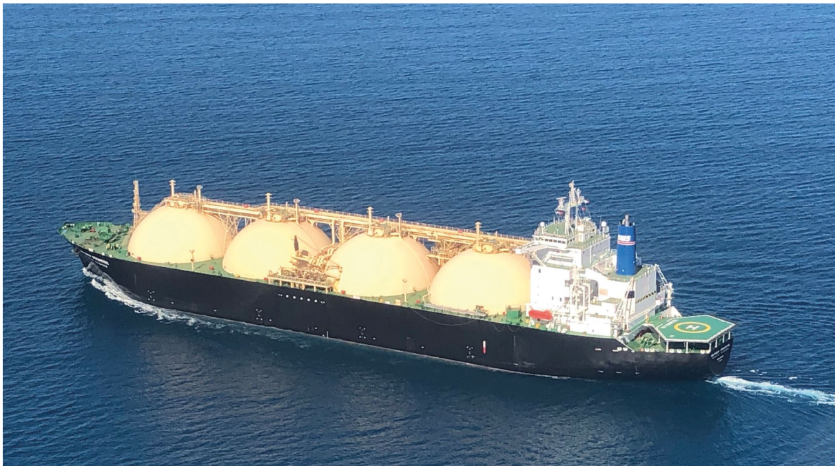
Figure 2.5: Gas tanker with purpose built helicopter operating and landing area at poop deck
