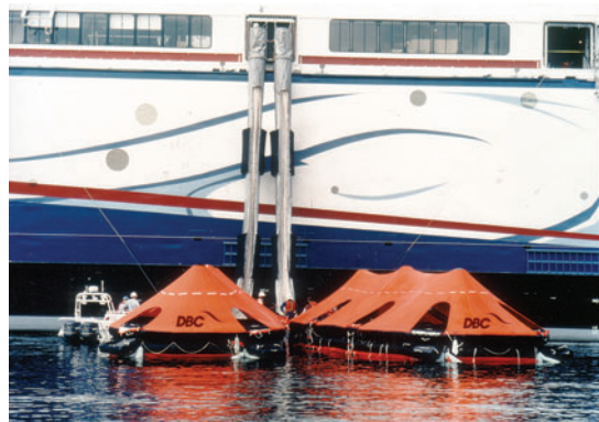
Figure 1.12 - Marine evacuation chute training exercise
