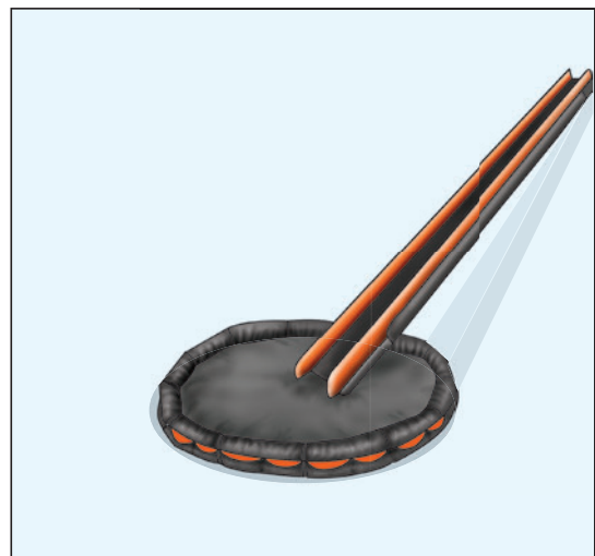
Figure 1.9 - Marine evacuation systems: single escape slide
