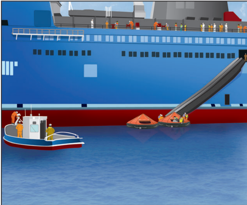
Figure 1.7 - Practical demonstration of the Viking Marine Evacuation System
