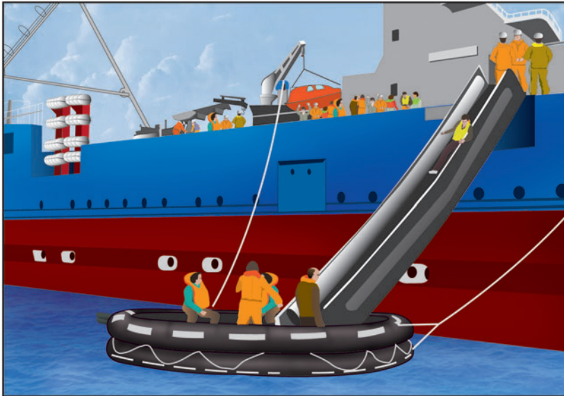
Figure 1.10 - Demonstration of the single trackway escape slide. Racked stowage of liferafts can also be seen, together with the single-arm davit rescue boat in a midships position.
