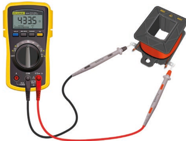
Figure 1.14a - Measuring contactor coil resistance
