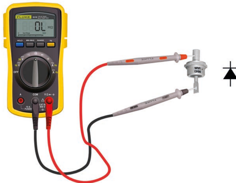
Figure 1.15b - Measuring PN junction resistance in reverse bias (positive lead is connected to cathode)
