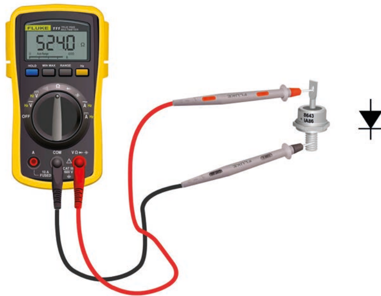
Figure 1.15a - Measuring PN junction resistance in forward bias (positive lead is connected to anode)
